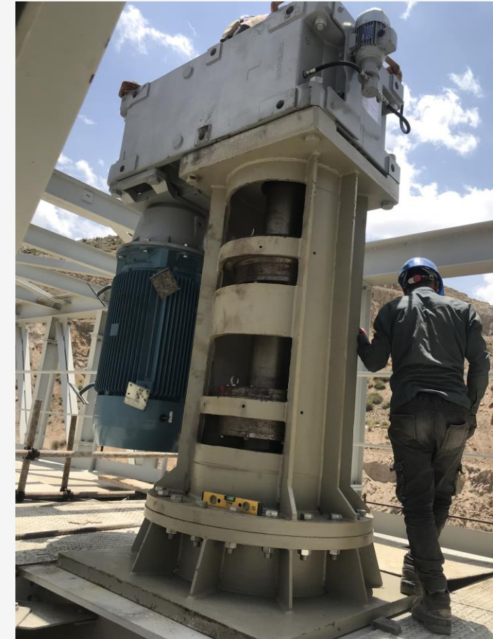
Copper Tailing Holding Tank 200kw, Impeller dia5.9m, Weight:19.5 ton
