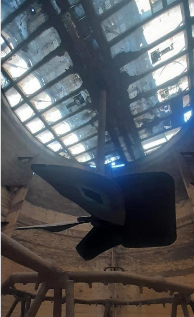
▲ Bioleaching Copper Reactor 110kw, 5.8m dia
